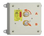
Key A is released from the key switch and the power supply is switched off. Key A is then inserted and turned in the DAE unit. Once turned, the time delay begins. Key B is held in the DAE until time elapses. Once the time delay has elapsed the indicator bar on the DAE rotates from red to white. Key B can now be turned and removed.
