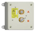
When the machine is running, key A is trapped in the key switch controlling the power. Key B is trapped in the mechanical time delay unit. This key is used to access the machine area, once machine has stopped running.
